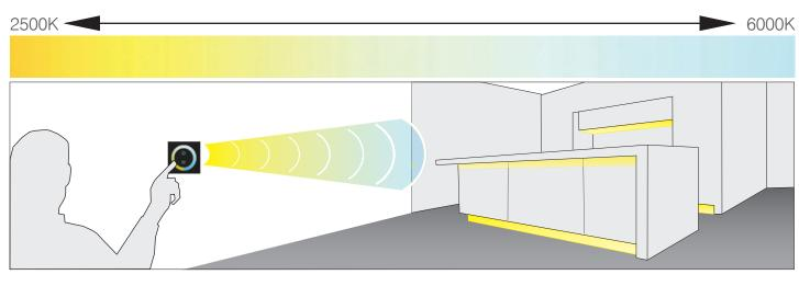
By the ingenius combination of two LED chips alonside each other, a colour spectrum of 2500K to 6000K can be achieved using a wall mounted or remote touch pad controller.
